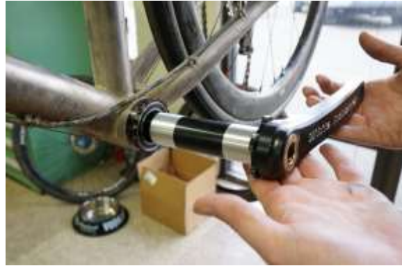
Fig.6 Installing spindle w/ arm in place.
