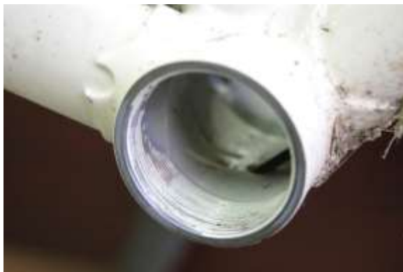
Fig.1 BB threads clean and ready for install.
