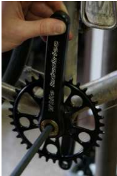
Fig.7 Crank arms clocked 180 degrees
