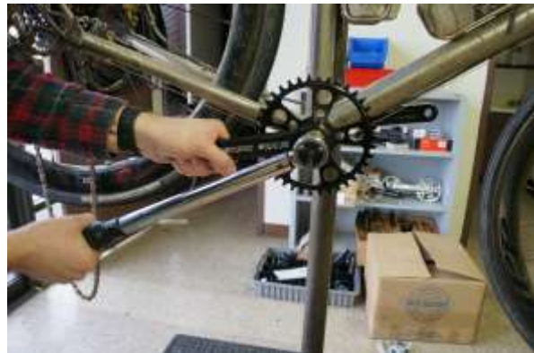
Fig.8 Torque to 50 Nm.
