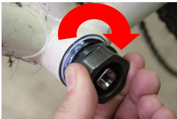
Fig.7 Tighten non-drive side cup, clockwise.
