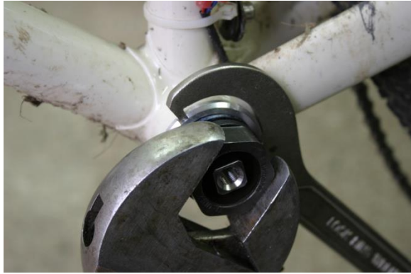
Fig.9 Hold cup while lock ring is tightened.
