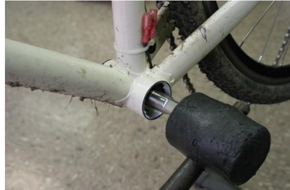
Fig.6 Gently tapping spindle into place.
