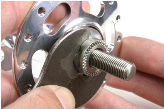
Fig.16 Wrench on flats of cone nut.
