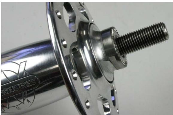
Fig.13 Axle is fully seated.
