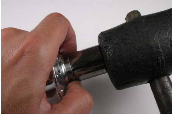
Fig.9 Tapping bearing into bore.
