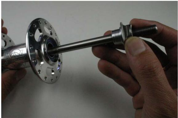
Fig.11 Installing axle assembly.
