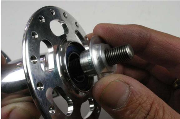
Fig.14 Installing aluminum cone nut.
