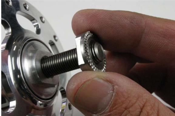
Fig.5 Remove lock nut.
