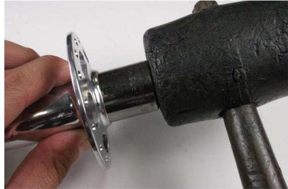
Fig.10 Fully seat bearing in bore.
