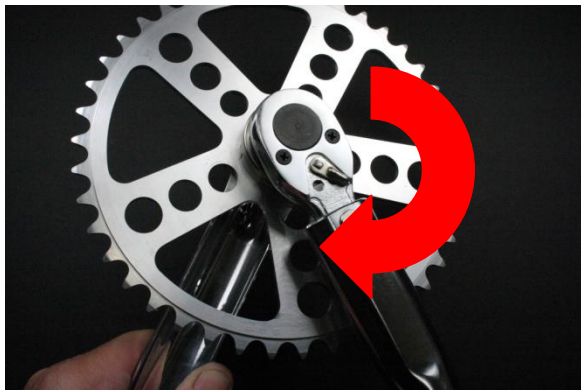
Fig.7 Tighten clockwise, 30 ft./lbs.
