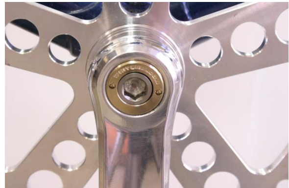
Fig.16 Bronze self-extracting ring installed.
