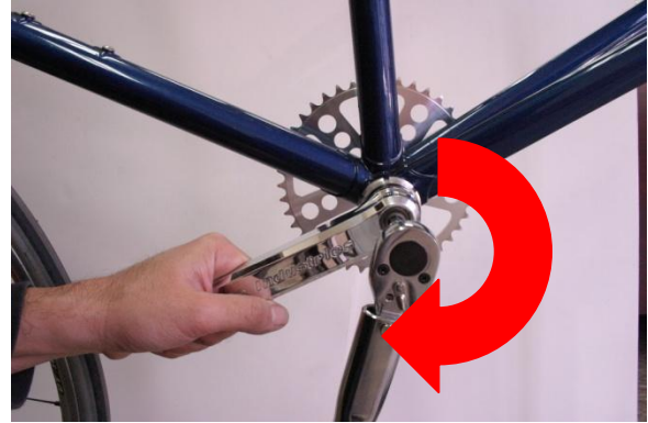
Fig.14..Tighten clockwise to 30 ft./lbs.
