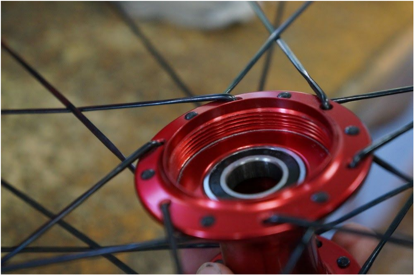
Fig. 6, Threads must be clean before installation
