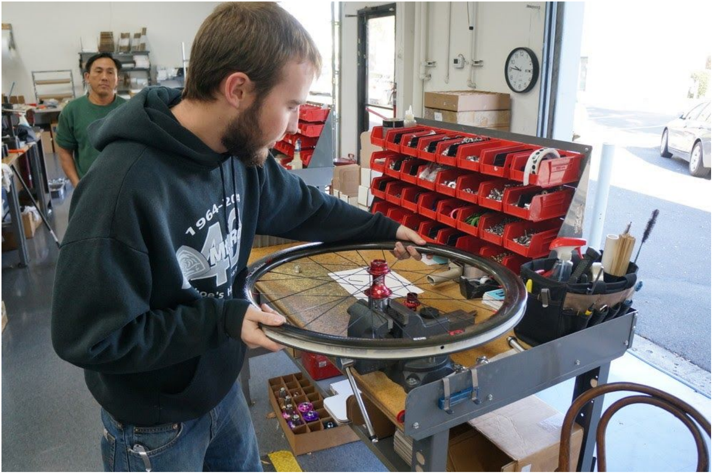
Fig. 5. Spinning the ring off the hub
