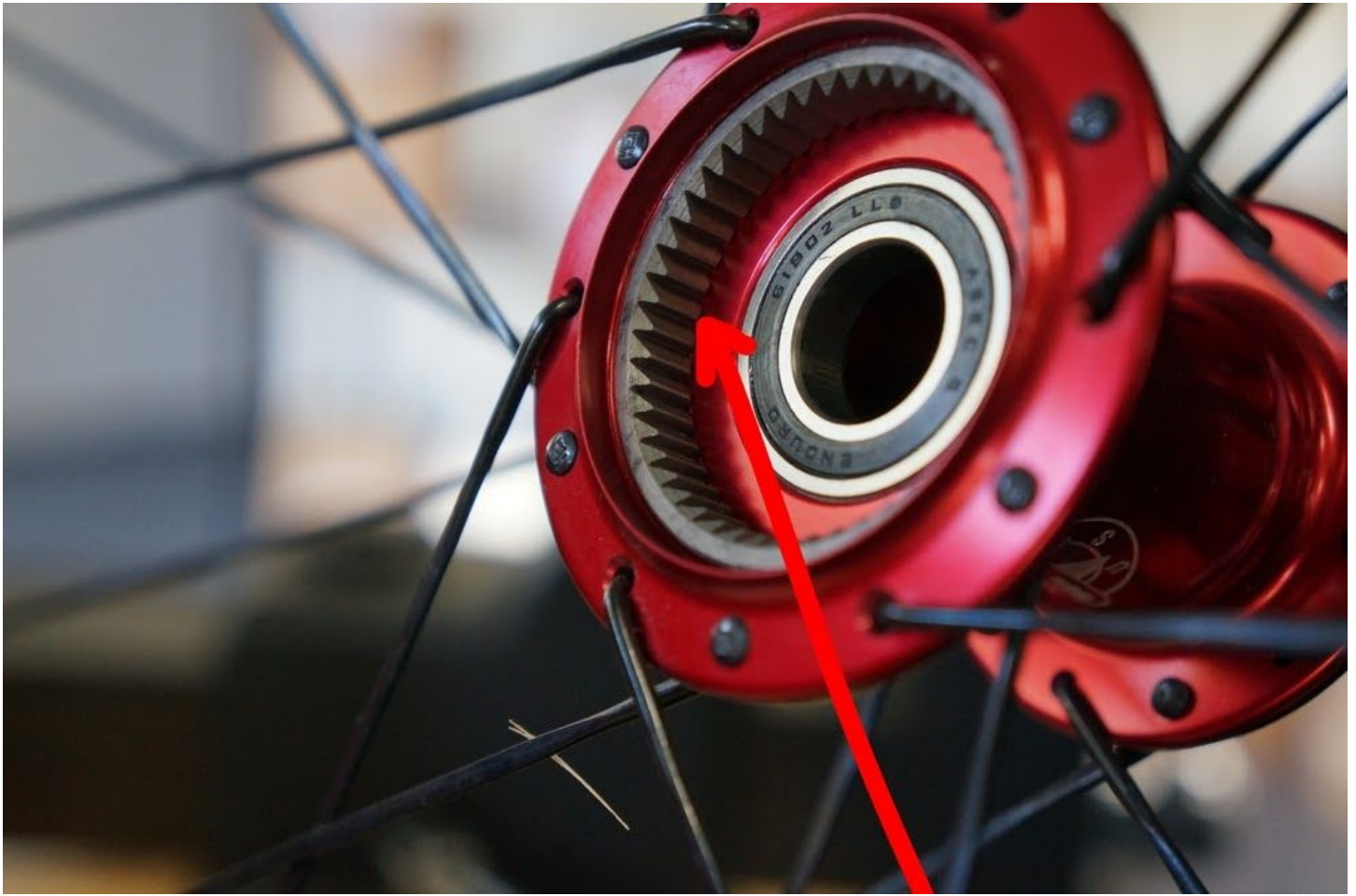
Fig. 8 Ratchet ring threads all the way down against the hub shell
