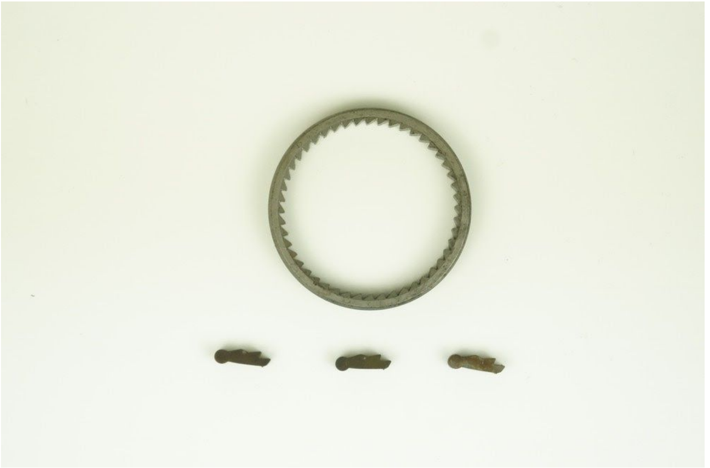
Fig 2, 48 tooth engagement pawls and ratchet ring. Note: pawl with two teeth at tip
