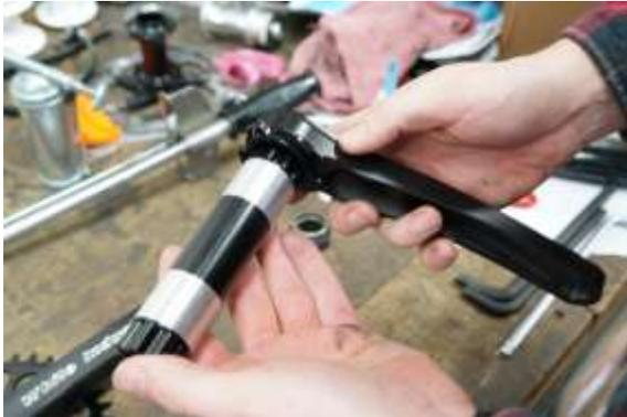
Fig.5 Mating spindle to arm
