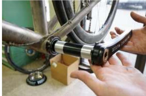
Fig.6 Installing spindle w/ arm in place.
