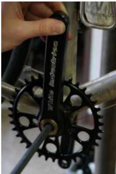
Fig.7 Crank arms clocked 180 degrees
