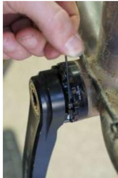
Fig.10 Cinch down adjustment ring
