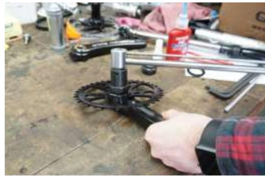
Fig.4 Tighten locking ring
