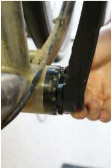
Fig.9 Adjustment ring placement.
