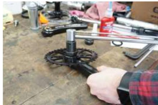
Fig.4 Tighten locking ring
