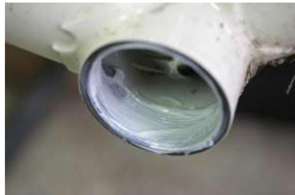
Fig.2 Greased threads.
