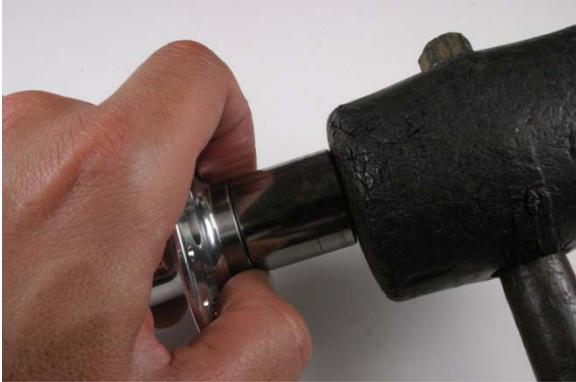
Fig.9 Tapping bearing into bore.
