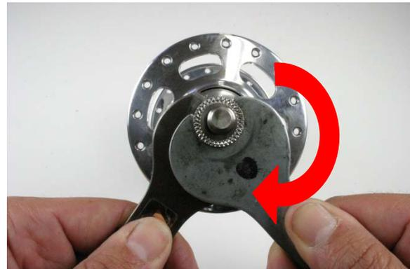
Fig.17 Hold cone nut and tighten lock nut.
