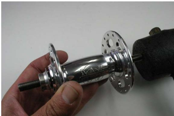
Fig.7 Tap axle assembly out of shell.
