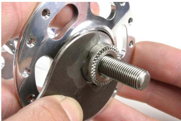
Fig.3 Fit cone wrench onto cone nut.
