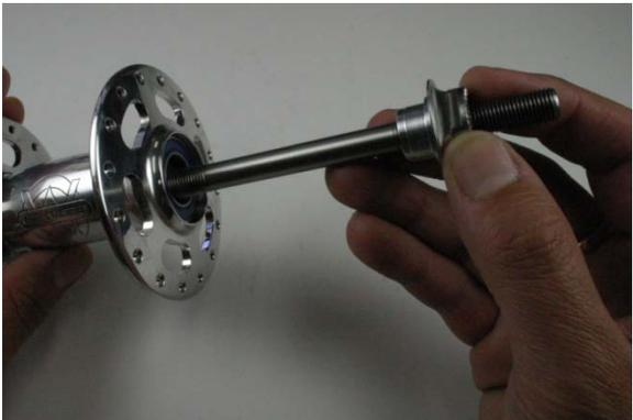
Fig.11 Installing axle assembly.
