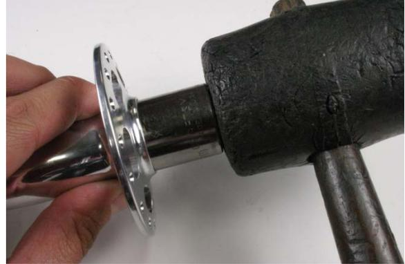
Fig.10 Fully seat bearing in bore.
