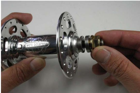
Fig.1. Removing axle nuts.
