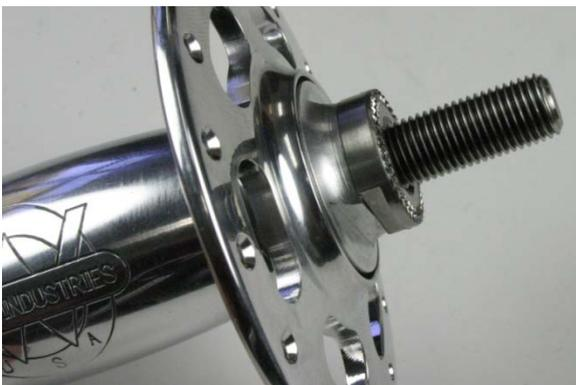
Fig.13 Axle is fully seated.
