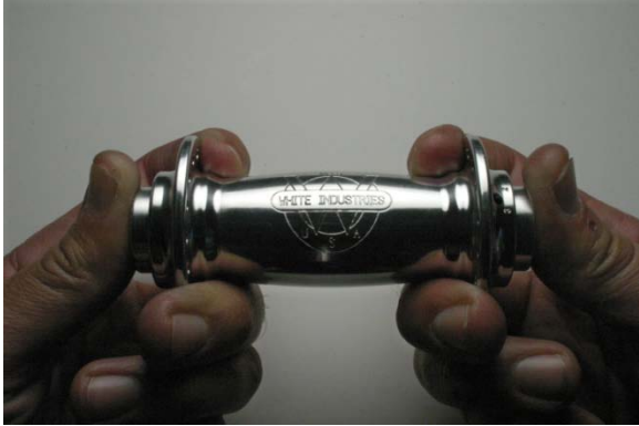
Fig.17 Checking for play in hub.
