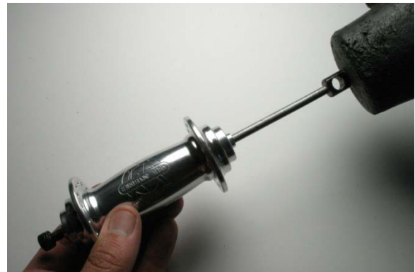
Fig.4 Tapping skewer to remove axle end.
