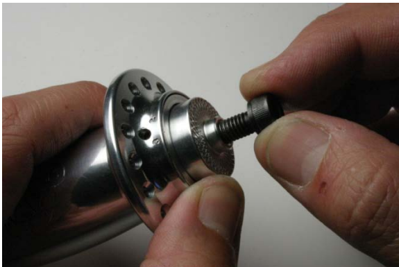
Fig.3 Threading in 6mm bolt.
