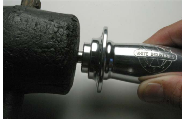
Fig.9 Tap axle end to fully seat.
