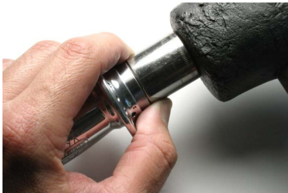
Fig.6 Tapping bearing into bore.
