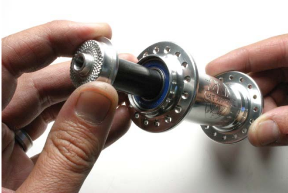
Fig.8 Installing axle with pressed on end.
