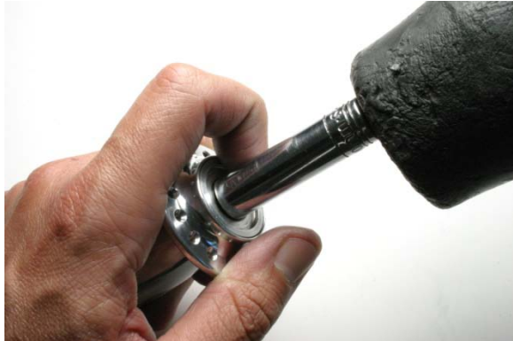
Fig.4 Tapping axle through hub shell.
