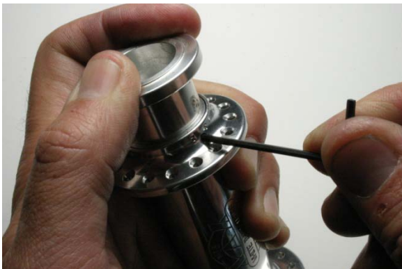
Fig.14 Slip tubing/socket over axle end.
