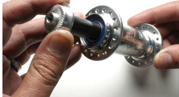
Fig.5 Removing axle from hub shell.
