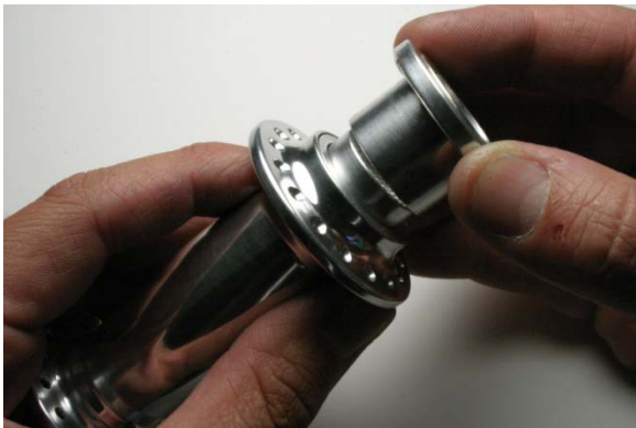
Fig.14 Slip tubing/socket over axle end.
