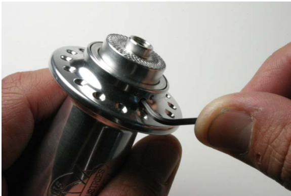
Fig.1 Loosening set screws.
