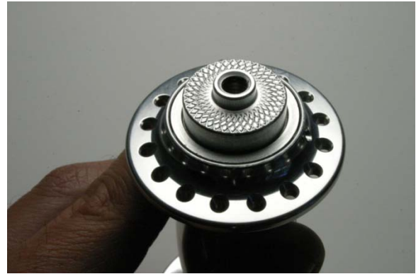
Fig.13 Axle end installed.
