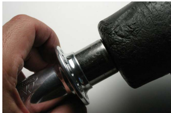
Fig.7 Fully seat bearing in bore.
