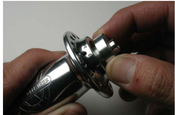
Fig.2 Removing adjustable axle end.
