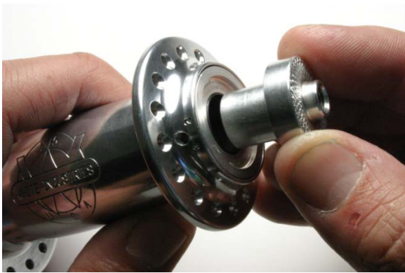
Fig.12 Inserting axle end.
