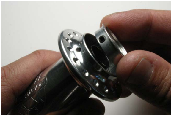
Fig.10 Installing adjusting collar.
