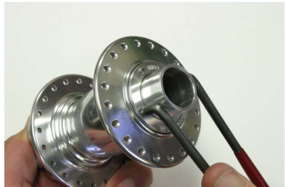
Fig.15 Tighten locking collar.
