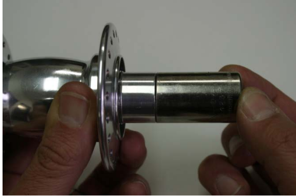
Fig.5 Butt socket up against axle.
