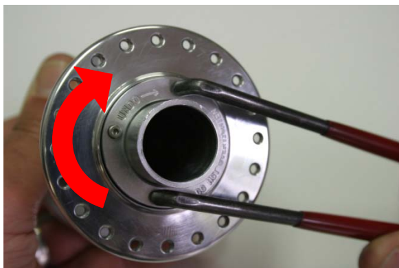
Fig.3 Turn lock ring clockwise to loosen.
