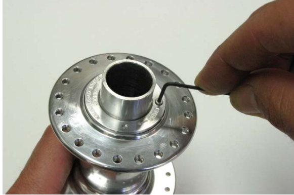
Fig.16 Tighten 1 ½ mm screw.
