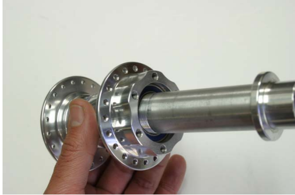
Fig.12 Insert axle on disc rotor side.
