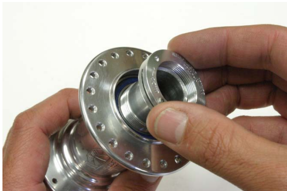
Fig.14 Installing locking collar.
