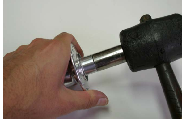
Fig.6 Drifting axle through hub shell.
