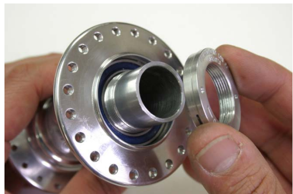
Fig.4 Removing lock ring.
