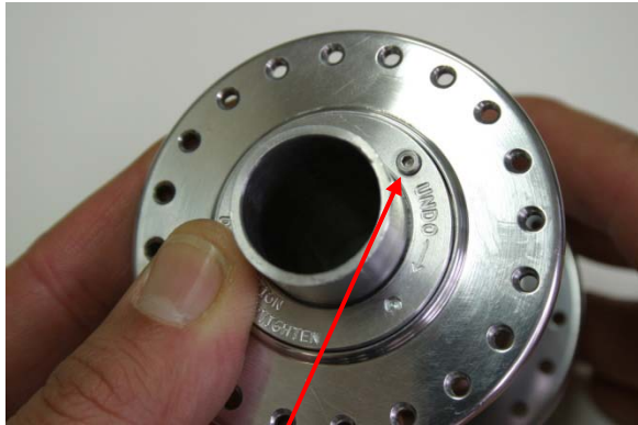
Fig.1 Screw location on locking collar.
