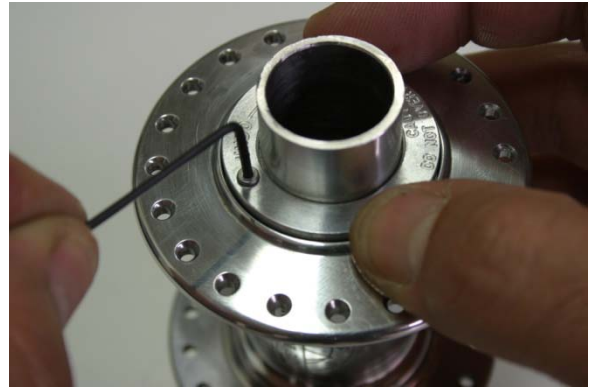
Fig.2 Loosen screw in locking collar.
