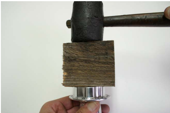
Fig.10 Gently tap bearing until flush with shell.
