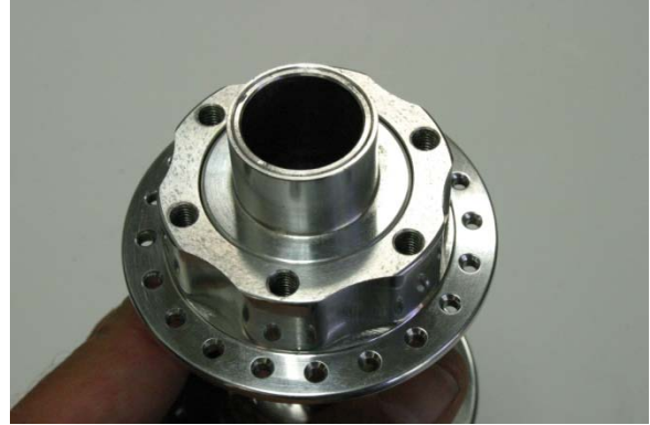
Fig.13 Axle fully seated in hub.
