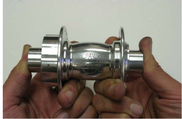
Fig.17 Checking for play in bearings.
