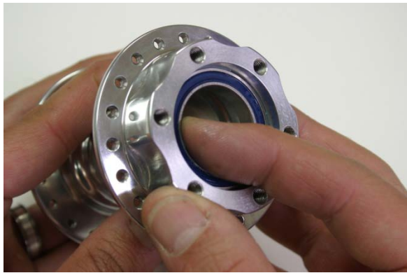
Fig.7 Checking bearings for roughness.
