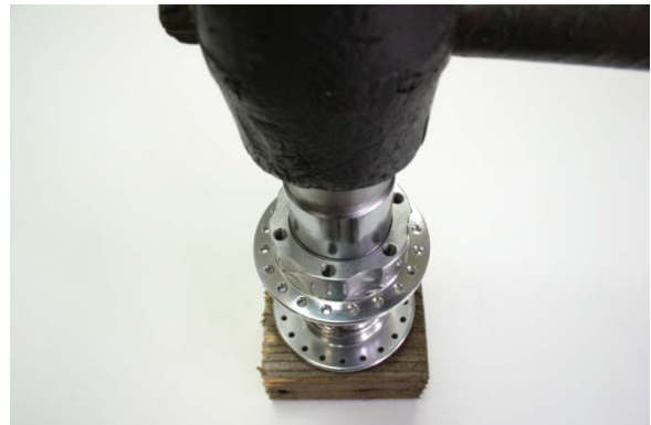
Fig.11 Use socket to fully seat bearing.
