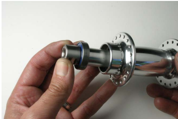
Fig.11 Removing axle/bearing assembly.
