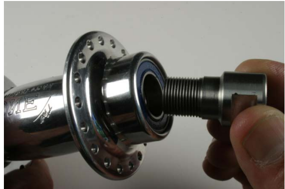
Fig.2 Removing axle end.
