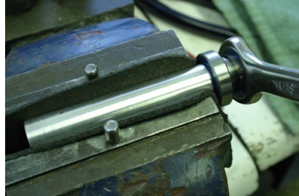
Fig.6 Axle in vise to remove axle end.
