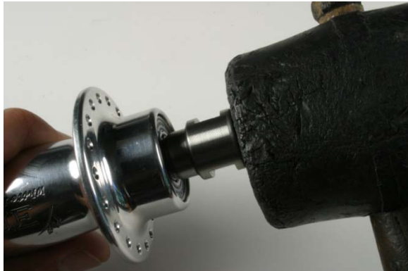
Fig.3 Tapping bearing out with mallet.
