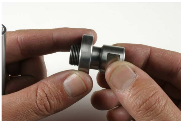
Fig.12 Placing bearing on axle end.
