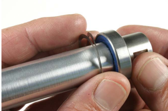
Fig.5 Washers between bearing and hub shell.
