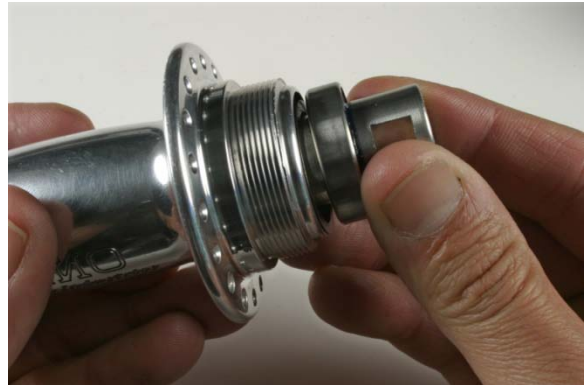
Fig.4 Withdrawing axle/bearing assembly.
