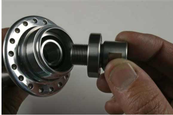
Fig.18 Installing axle end and bearing.
