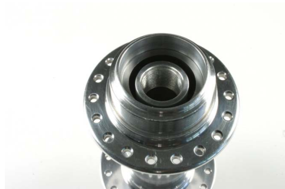
Fig.17 View of washers on shoulder.
