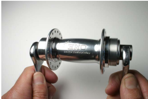
Fig.20 Tighten axle ends with wrenches.
