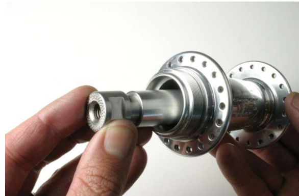
Fig.8 Axle going into hub shell.
