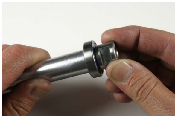
Fig.13 Threading axle end into axle.
