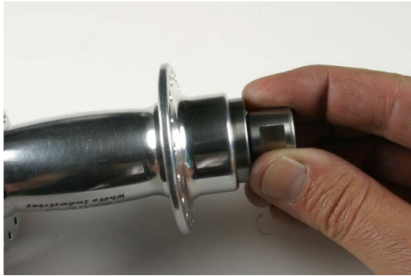
Fig.14 Starting bearing into bore.
