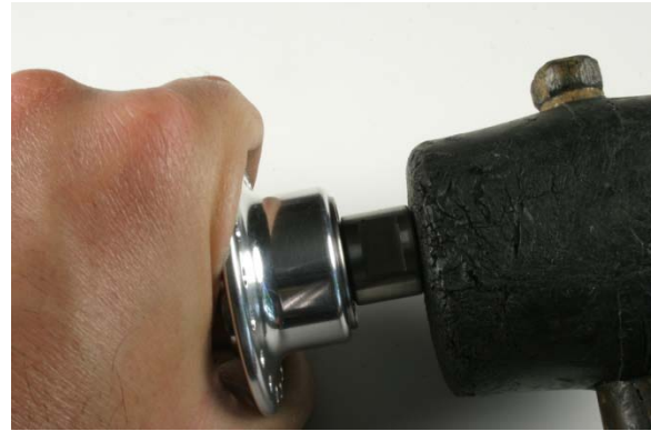
Fig.15 Tapping bearing into bore.
